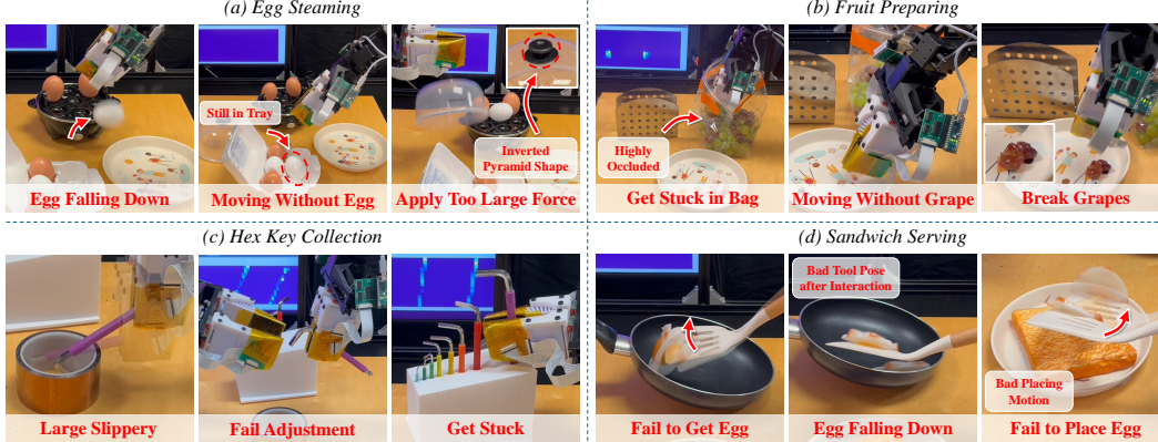
Figure 13: Failure Cases. We present typical failure cases of the baseline method for all four tasks and analyze the reasons for these failures to highlight the complexity of the tasks and the importance of tactile feedback during these steps.
