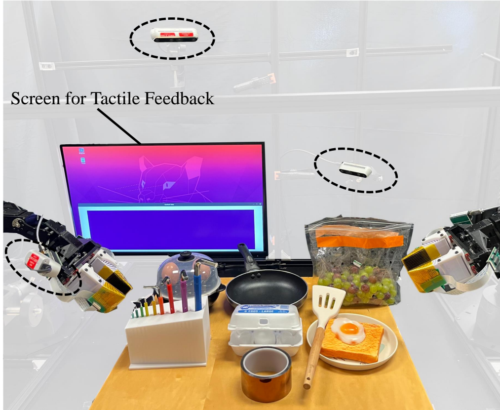
Figure 12: System Overview. We attach four tactile sensors to four robot fingers and install three Realsense cameras to cover the workspace. All the objects used for the task are shown in the workspace. Additionally, we install a background screen to display the tactile feedback.
