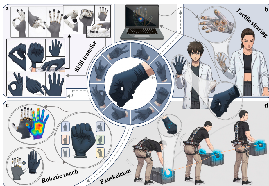
Fig. 1. Design concept and potential application scenarios of the bio-inspired hierarchical flexible fabric glove. a Robot skill learning and transfer based on tactile demonstrations; b shared tactile feedback through cross-end conversion of full-palm pressure signals; c full-palm tactile input for robotic dexterous manipulation; d hand-contact intention sensing for exoskeleton assistance control.
